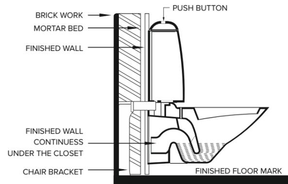
1. If the wall is going to be plastered for a thickness of 12 mm and a tile thickness of 6-7 mm, the projection of the bolts from the finished wall should be 66 mm only.
